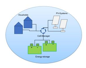
The current simulation runs as follows: Every second the power components send their consumption quantity or generation capacity to the cell manager on a regular basis. The cell manager in turn calculates the total consumption and generation, creates a schedule based on the merit-order-method and sends this to the respective energy producers. They execute the schedule via the physical connection.
