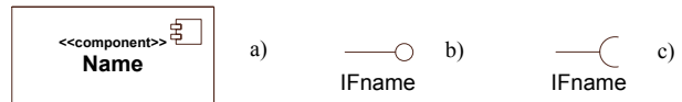
Figure 4. Building blocks of a component diagram: a) component with name "Name" b) provided interface with interface name "IFname" c) required interface with interface name "IFname"
