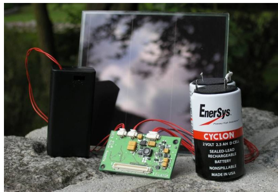
Fig. 2. Solar power module for an iris node with emergency battery, solar panel, electronics with node adapter and rechargeable lead batteries.
